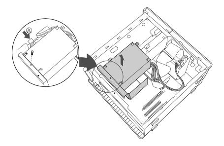
4 Rotate the power supply upside down and rest it on top of the chassis where the hard drive is located.
